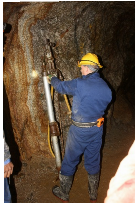
Photo:- Demonstrating use of rock drill
