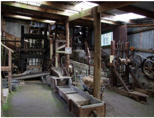
Photo:- Kelly Mine - Processing mill with Californian and Cornish stamps plus washing strips
