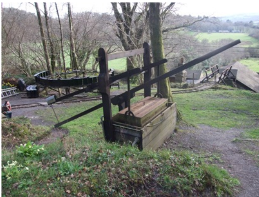
Photo:- Kelly Mine - Jigger box for ore washing
