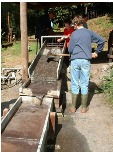
Photo:- Kelly Mine - Jigger box for ore washing
