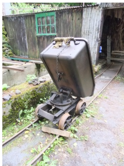
Photo : Steel tram showing safety catch
