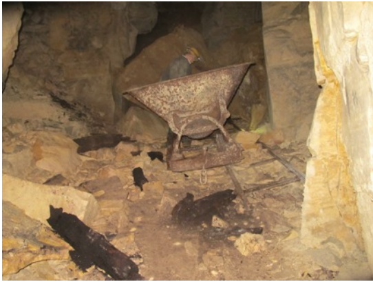
Photo: V-tipper wagon and track section in LBG
