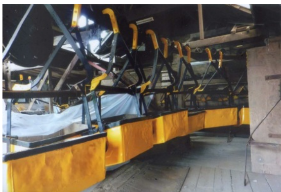
Photo 3. Proudly re-painted, these buckets stand ready for their return from the quarry, each holding 290kg of quarry waste.
