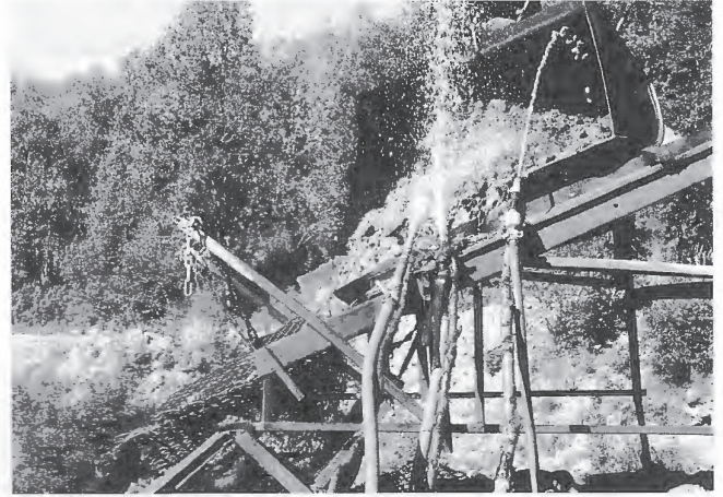
Detail showing the water jets that flush out the shovel
